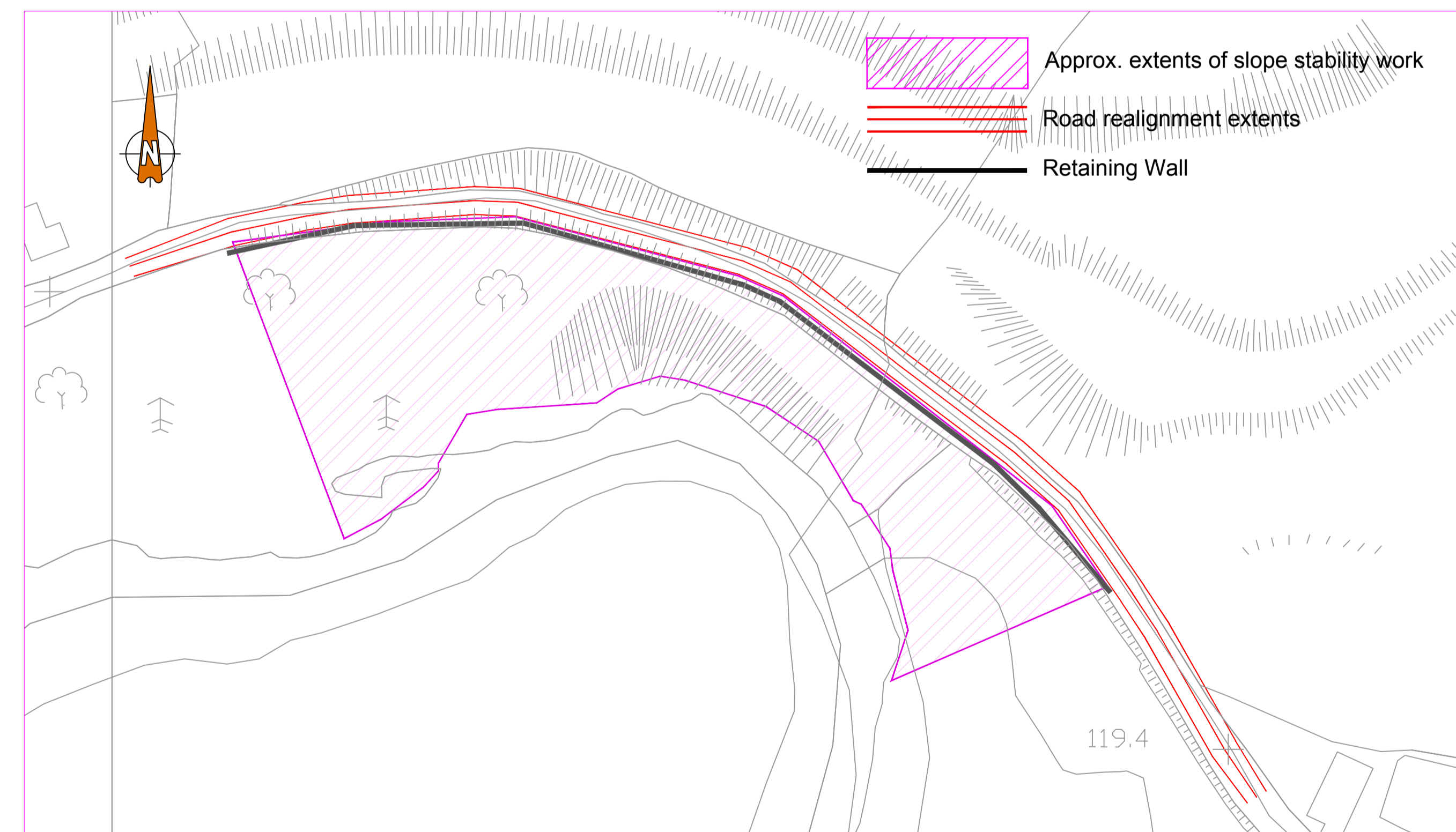
Option D: Existing alignment of L6048 maintained with introduction of piling and retaining wall on southern side of the road. Slope of 1:2 to be introduced to run towards the River Liffey. Existing road alignment maintained with 300m re-build of existing road build up.
